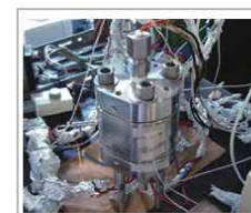
Batch-type film-deposition system using supercritical CO 2 fluid
